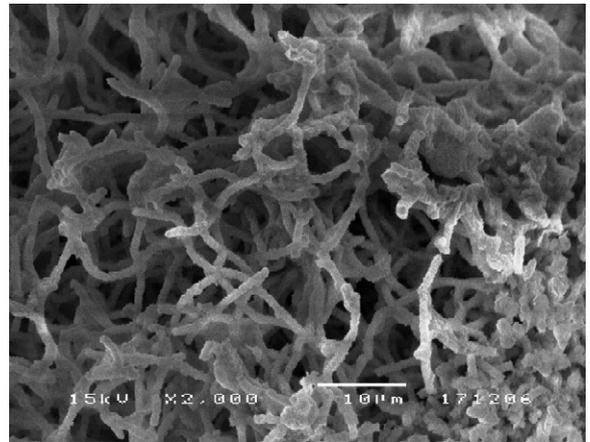
Fig. 17. SEM micrograph of the tube fragments showing iron oxides and ferruginous clay with a particular morphology, as intricate filaments like balls of thread or rod, located in the pores between sand grains.
