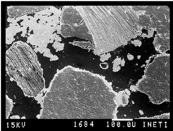
Fig. 12. SEM micrograph of the exterior band of the tubes showing a coarser structure with sand grains covered by a thin film of iron oxides and ferruginous clay, separated by empty pores.
