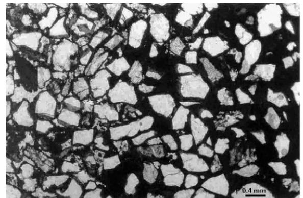
Fig. 11. Optical micrograph of the intermediate and inner parts of the tubes showing a gradual iron oxide enrichment and ferruginous clay represented by cement thickness involving the grains.
