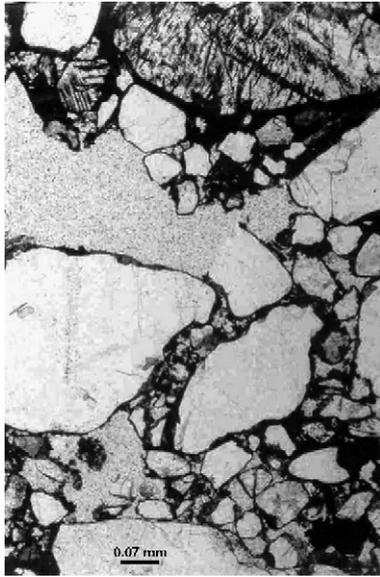
Fig. 9. Optical micrograph of exterior part of the tubes showing large quartz grains coated by a thin film of iron oxides and ferruginous clay and the empty pores between them.
