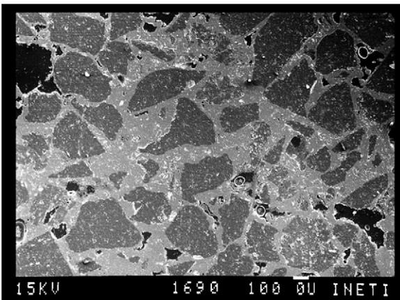
Fig. 13. Massive and compact aspect of the inner part of the tubes by almost complete infilling of the pores by iron oxides and ferruginous clay (SEM micrograph).
