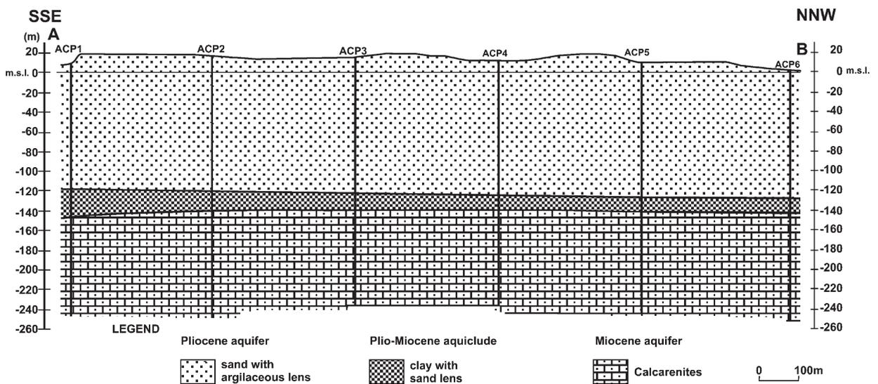
Fig. 18. Schematic geological section of the Tagus-Sado aquifer system in the Mitrena Peninsula, 7 km eastwards of Setúbal Peninsula (Mendonça et al., 2003).
