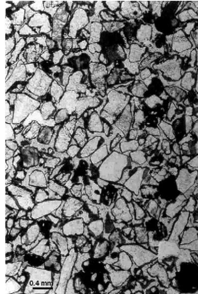
Fig. 10. Optical micrograph of exterior part of the tubes showing large quartz grains coated by a thin film of iron oxides and ferruginous clay and the empty pores between them.
