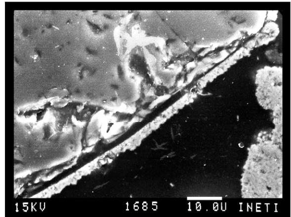
Fig. 14. Detail of a sand grain showing an empty space between the grain surface and the iron oxides and ferruginous clay coating (SEM micrograph).
