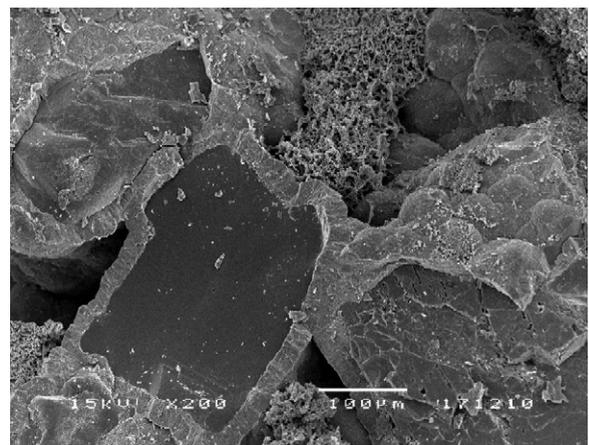
Fig. 15. SEM micrograph of the tube fragments showing sand grains completely surrounded by iron oxides and ferruginous clay coating with a fibrous fabric.
