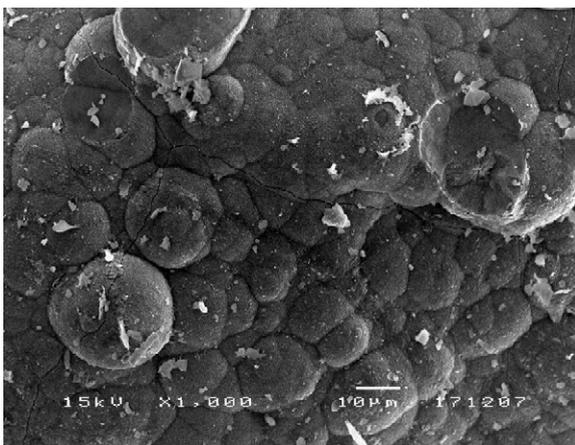
Fig. 16. SEM micrograph of the tube fragments showing a botryoidal aspect of the iron oxides and ferruginous clay on the external face of the coating.
